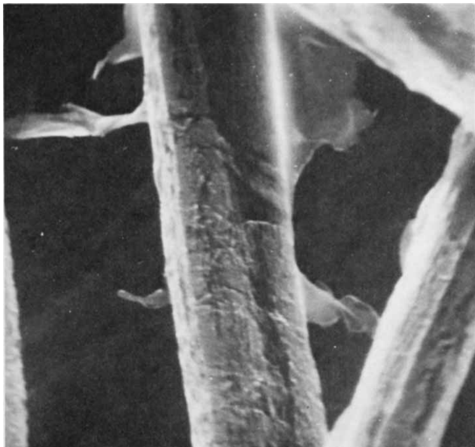
Fig. 15. Sisal primary walls, appearing as "flakes" during ultrasonic disintegration.
